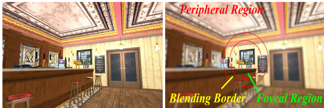
Fig. 8: Application of our gaze prediction to gaze-contingent rendering. Left: Rendered in normal mode; Right: Rendered using gaze-contingent rendering mode. Gaze-contingent rendering decreases rendering quality in the peripheral region while maintaining high fidelity in the foveal region. The inner circle is the foveal region rendered with high quality, the outer region is the peripheral region rendered with low quality and the blending border denotes the transitional region.
